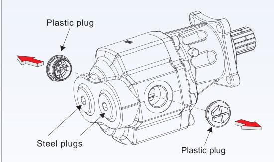
**REMOVE THE 2 PLASTIC PLUGS BEFORE START-UP.** Steel plugs can be fit in the side ports when using rear inlet/outlet.
